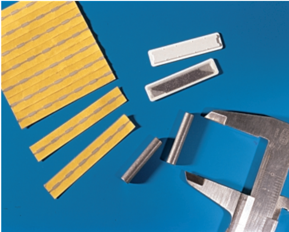
Fig. 7: EAS-tags with strips of SENSORVAC and rods of SEMIVAC.
